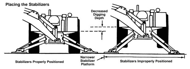
Set the stabilizers to remove weight from the rear wheels. The wheels are to remain touching the ground as this provides for the widest stabilizer stance and the lowest center of gravity. Raising the wheels off the ground will not only reduce stability and digging depth, but will impair performance and impose unnecessary stress on the unit.
